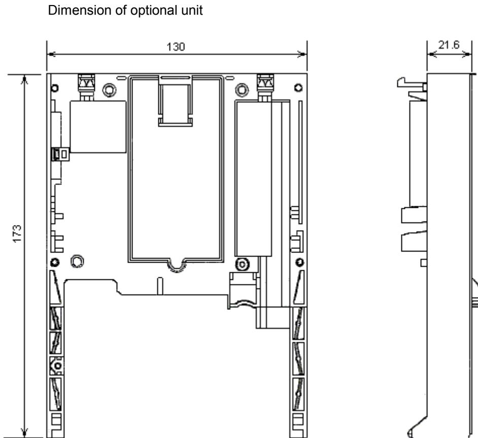
The control panel depth increases about 21.6mm when the option is installed. Secure the front space from the inverter control panel fully. The space which is necessary for the option installation varies in the inverter capacity rate. Please refer to the inverter instruction manual.
